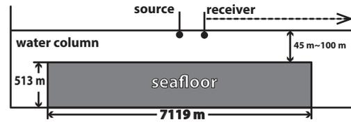
Figure 3: Physical modeling geometry. Offset range:  $200 \sim 3500 \text{ m}$ , Receiver interval:  $10 \text{ m}$ . Two different water depths are simulated:  $45 \text{ m}$  and  $100 \text{ m}$ . The dashed line arrow indicates the moving direction of the receiver.
