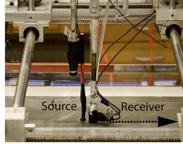
Figure 2: The physical modeling system used for marine guided-waves modeling. The gantry, source and receiver, plus model are shown. The source is placed in the center of the block and receiver is moved away from the source. The dashed line arrow indicates the moving direction of the receiver.
